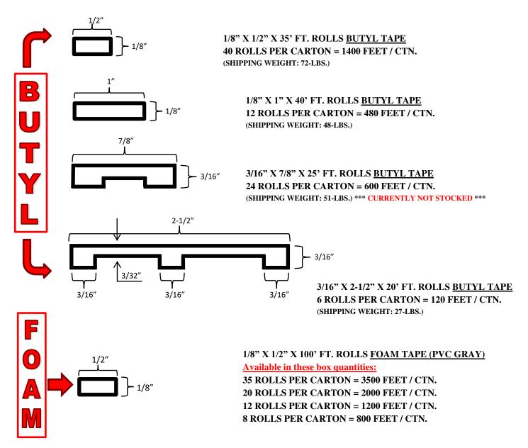
\*The above sizes for both Butyl and Foam Tape are the most common sizes utilized in the metal industry.
