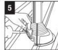
Apply sealant to the underside of the base. Shape Retrofit to roof by pressing the aluminum base to the roof contours.
