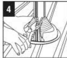
Squeeze Gripper tightly with pliers to crimp, start at the top and work down to the base.
