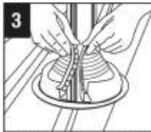
Wrap Retrofit around pipe, join the interlocking teeth starting from the top and proceeding down.
