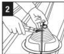
Using tin snips, cut the flashing to fit pipe, starting opposite the Gripper.
